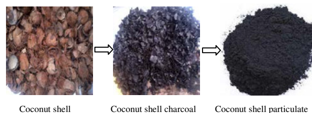
Figure 1. Production process products: coconut shell – coconut shell particulate
