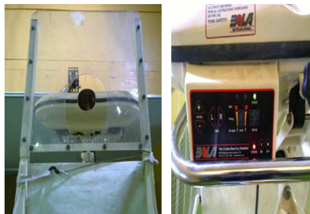
Figure 1. Front view of the bowling machine (left) and the control module located at the back of the machine (right)
