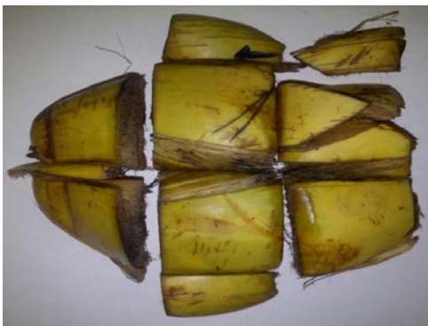
Figure 13. Final product from cutting machine (0 days old, faced downward, cut parallel to blade)
