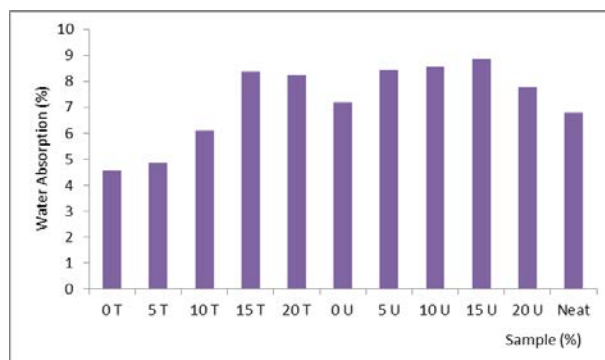
Figure 7. The Rate of Water Absorption for the Developed Composites and the Neat sample after 7 Hours of Immersion
