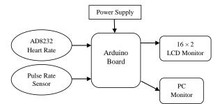
Figure 1. Functional Block Diagram of the Device
