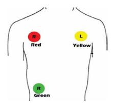
Figure 2. The placement of AD8232 ECG Sensor on human body
