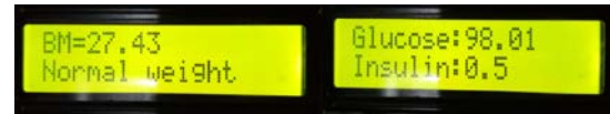
Figure 6c. Result of Measurement Displayed on LCD of BMI, Glucose and Insulin computed
