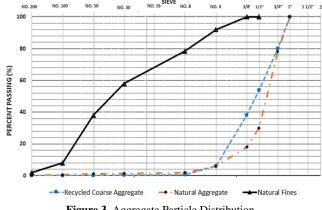
Figure 3. Aggregate Particle Distribution
