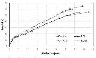
Figure 10. Load vs Average Deflection for Concrete Beams
