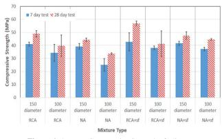
Figure 6: Average Compressive Strength of Mixtures
