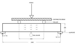
Figure 4. Third-point Loading of Reinforced Beam with 9 Demec Points
