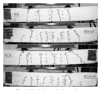
Figure 8. Cracking Patterns for Concrete Beams
