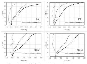
Figure 9. Load vs Strain Curves for Concrete Beams due to Flexural Loading
