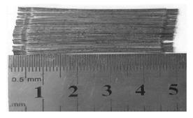
Figure 1. Dramix ZC 50/50 End Hooked Steel Fibers
