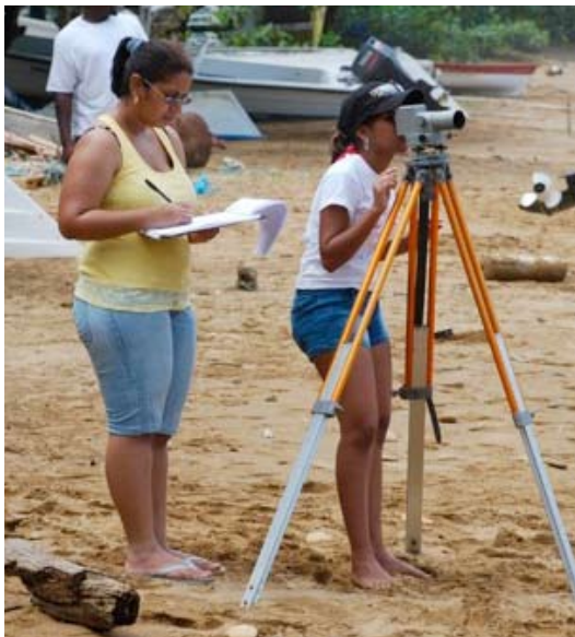
Beach profile surveying: Cristal Narine looks through the level, while Tamara Goberdhan takes notes.
