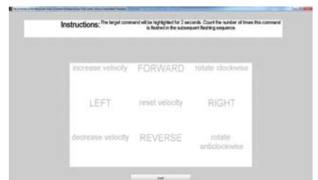
PICTURE 4 Screenshot of the Stimulus Presentation Paradigm users view during BCI usage
