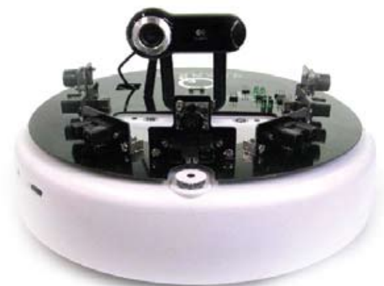
PICTURE 3 Quanser Qbot Autonomous Vehicle
