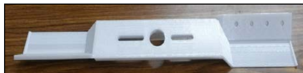
Figure 6. 3D-printed blade with support material removed
