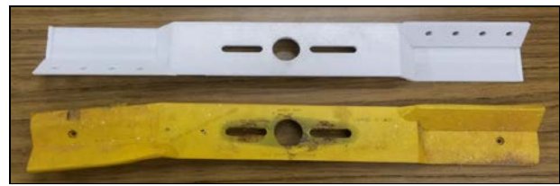
Figure 7. Original and redesigned lawnmower blades
