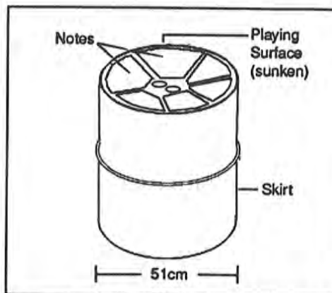
Figure 1: Typical Physical Attributes of a Cello Steelpan Component
