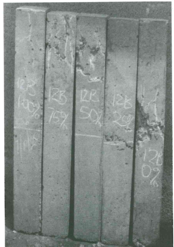
FIGURE 8: Failure Patterns of Bamboo Columns with Varying Laterite Content
