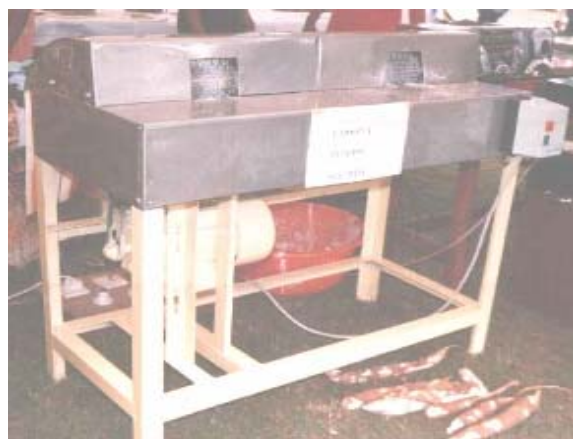
Figure 1(a). Double gang cassava peeling machine
