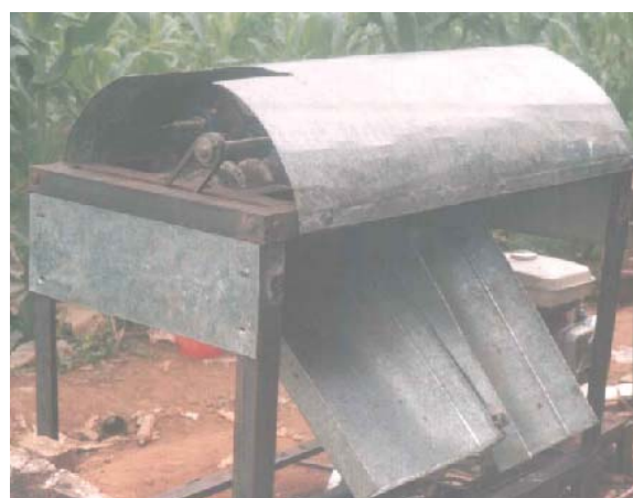
Figure 2. Self-fed cassava peeling machine
