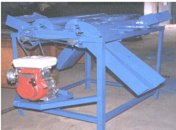
Figure 3. Double action self-fed cassava peeling machine
