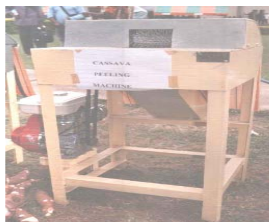
Figure 1(b). Single gang cassava peeling machine
