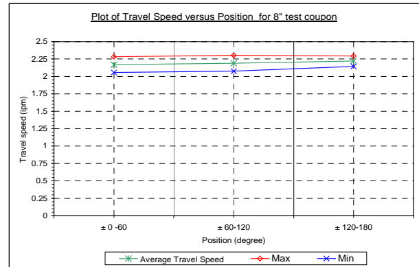
Figure 6. Plot of travel speed versus weld position for the 8" test coupon
