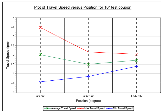
Figure 9. Plot of travel speed versus weld position for the 10'' test coupon
