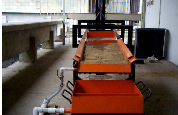
Figure 2. Soil erosion measuring facility with soil before testing
