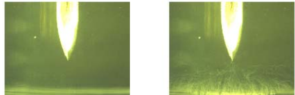
Figure 6. Sample colour electrical tree images
