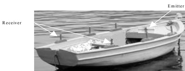
Figure 2. An RB with emitter and receiver
