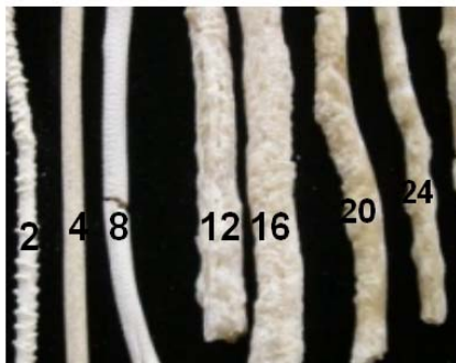
PLATE 3: Wheat Flour @ Moisture Content 30% & Screw speed 100 rpm arranged in order of duration of operation 2-24 minutes.
