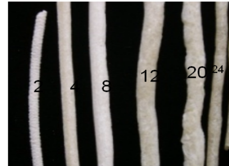
PLATE 6: Maize Starch @ Moisture Content 40% & Screw speed 100 rpm arranged in order of duration of operation 2-24 minutes.
