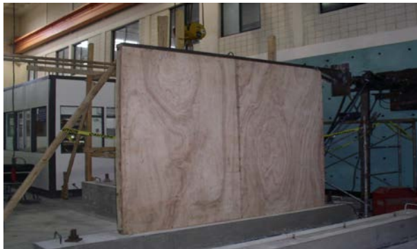
Figure 2. Shear-wall Test Setup
