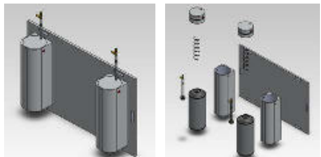
Figure 11. The Major Sub-Components of the Flame Pack in both the Collapsed and Exploded States
