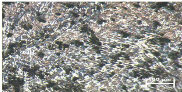
Figure 1. Microstructure of TWDI showing carbide precipitate Source: Ochulor et al. (2015)
