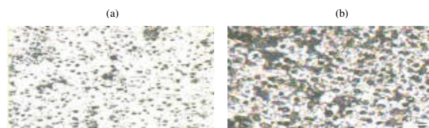
Plate #19: Optical micrograph of 2mm thick section (a) unetched (b) etched of D5
