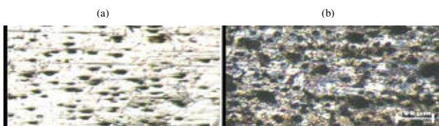
Plate #12: Optical micrograph of 4mm thick section (a) unetched (b) etched of D3
