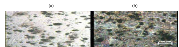
Plate #8: Optical micrograph of 3mm thick section (a) unetched (b) etched of D2
