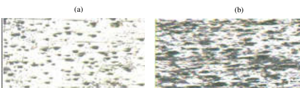
Plate #21: Optical micrograph of 4mm thick section (a) unetched (b) etched of D6
