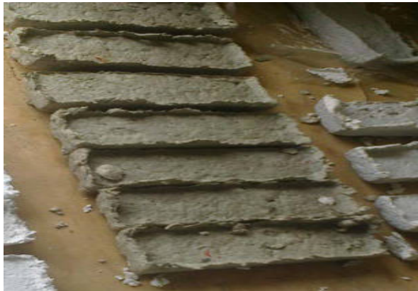
Figure 1. Samples of compacted brown paper samples mixed with natural rubber
