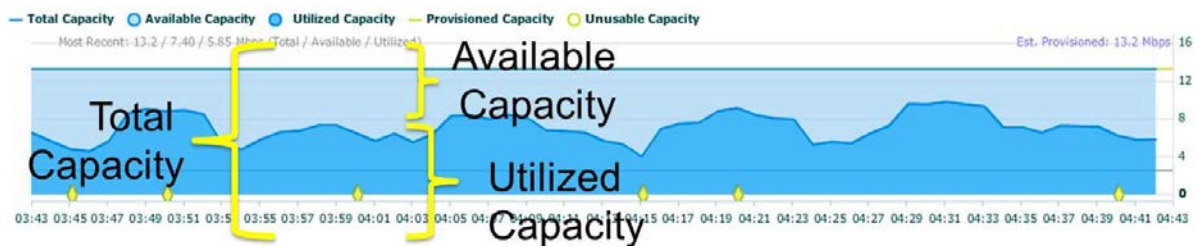
Figure 1. Illustration of the relationship between (total) capacity, utilised capacity and available bandwidth (capacity) Source: Abstracted from AppNeta (2012)
