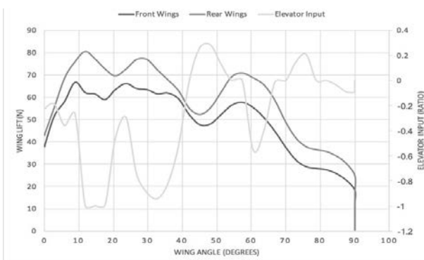
Figure 16. 2nd Transition Lift Forces wrt Wing Angle
