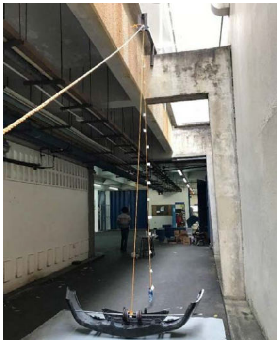
Figure 2: Image of simulated accident testing setup
