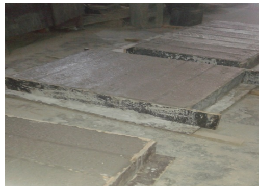
Figure 3. Beams for flexural strength test
