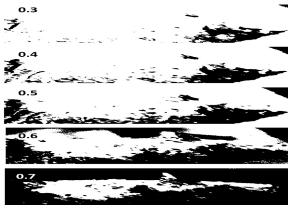
Figure 5. Impact of Level Value on Binarisation Process of Image 2
